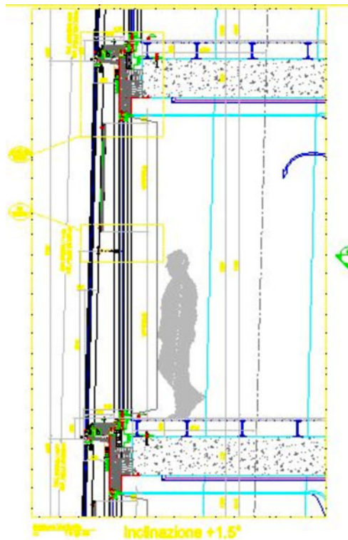
Fig. 1 Section of personalized curtain wall.
