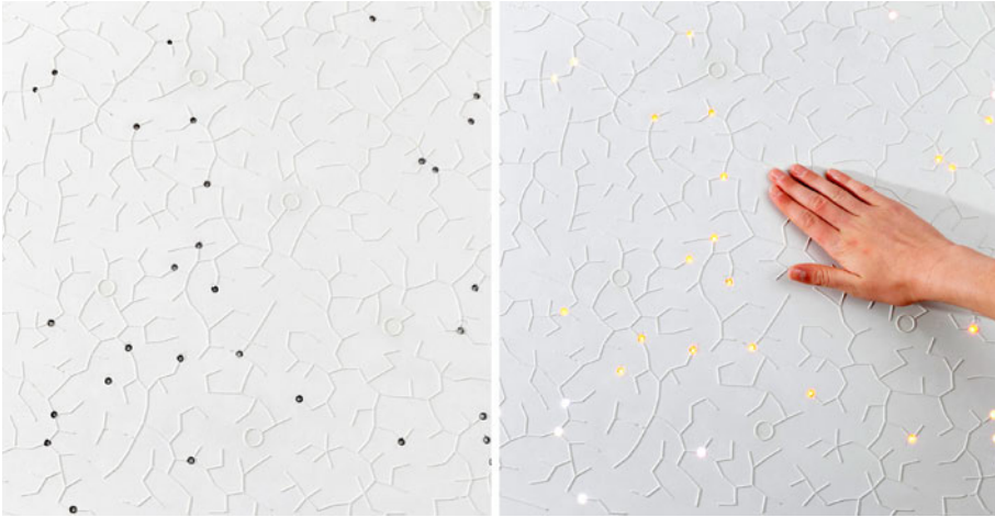
Fig. 4 Smart Concrete panel (in collaboration with CEA).
