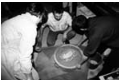
Sieving of earth to exclude too big pieces
